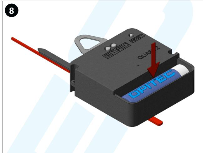
Insert the battery with the correct polarity and hang the clock in the desired location. The best reception properties are achieved when the clock face is facing Frankfurt/Main.
