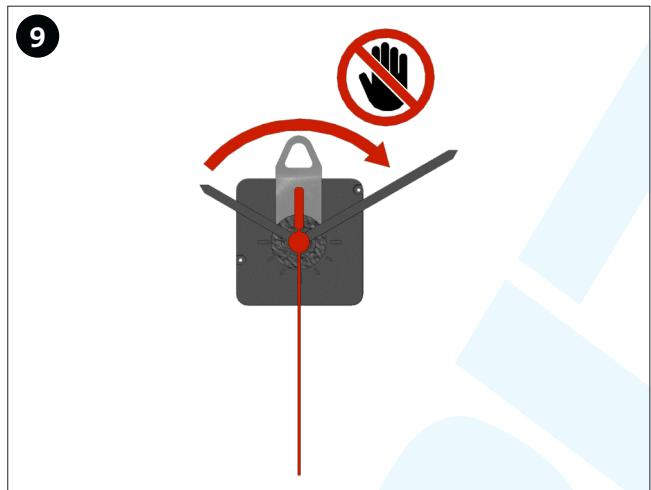
The clockwork begins synchronization with the DCF77 transmitter. The hands complete a few revolutions, stop for a while and then adjust to the correct time. Do not move or stop the hands by hand during this time!
