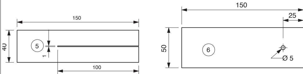
6.1.4 Glue the plywood parts (5) and (6) to the sides of the pine block (4) to form the sound box.
