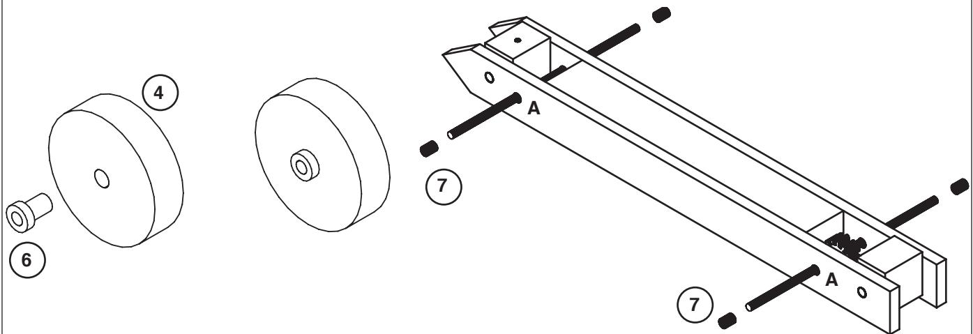
6.2.3 Insert and glue a brass bearing tube in each hole marked 'A' in the chassis side (2).
