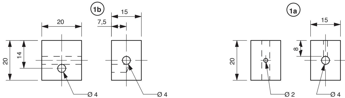
6.1.4 Then insert a dowel as an axle into each block (1a) and (1b).ensure that they are in the middle and then glue them in position.
