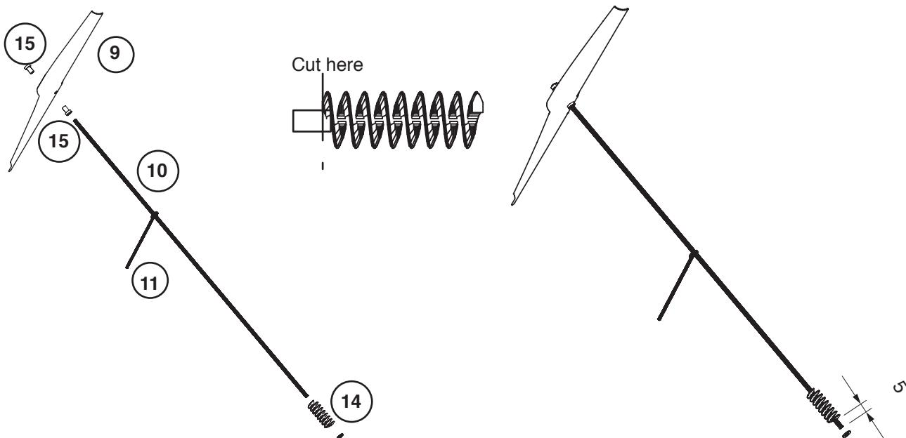
6.3.6 Place a washer (12) on the end of the shaft (10) after the worm (14) and then insert the end of the shaft and the support into the holes in parts 1a and 1b ( both of these blocks should be moveable)
