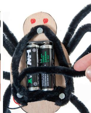
30 Loosen the other machine screws and clamp the pipe cleaner under them as shown (re-tighten) Then thread the remaining pipe cleaner over the battery case as shown
