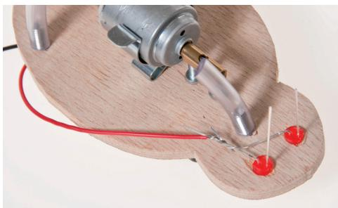
16. The red cable from the battery holder is joined to the Anode of the LEDs as shown . Twist it in place.
