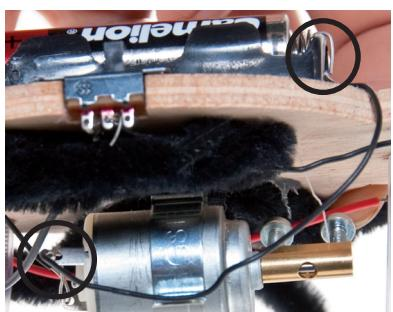
24. Cut a 60-70mm long piece of cable.(8) strip the ends Join one end to the free connections on the motor (6) The other end is connected to the minus pole of the battery holder ( Spring )
