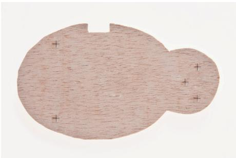
1. Trace out the outline of the spider using the pattern on page 5. Mark out the holes and use a bradawl to mark the centres. Cut out the shape of the spider and sand to finish.
