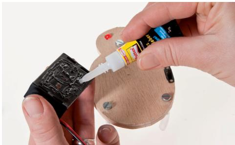
13. Coat the battery holder with an all-purpose glue
