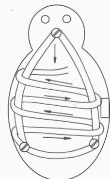
31. Once you have adjusted the PVC tubes and switched on the spider will either turn in a circle or walk backwards. This can be adjusted by moving the PVC tubes or the machine screws
