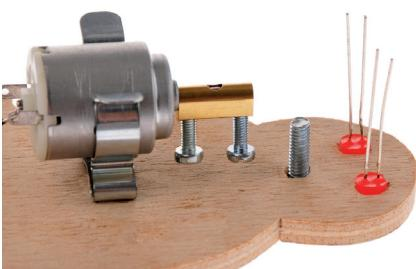
10. Take care when inserting the LEDs as they are poled. The longer legs should face together on the inside and the shorter legs toward the outer edge of the spider. As a second check the small flat on the edge of the LED also faces the outside
