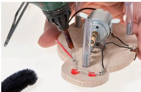
21. Bend the pipe cleaners in half and glue them in place as shown. Use a hot glue gun
