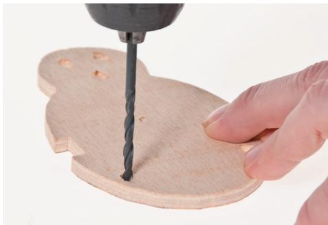
2. Drill the holes for the eyes, 5mm dia. See pattern on page 5. Drill the three holes for the legs. Now is the time to paint the spider if you wish.
