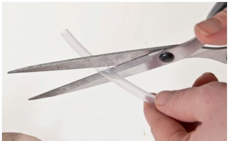
11. Cut three ca. 40mm lengths from the PVC tube (3). Then cut the ends of these at 45 degrees on one end .
