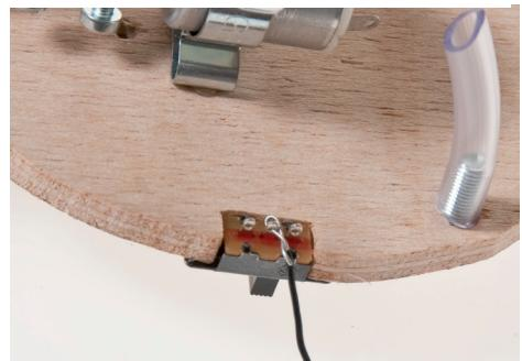
15. Cut a 80 mm length from the cable. Strip the insulation from the ends, join one end to the middle connector on the micro switch .
