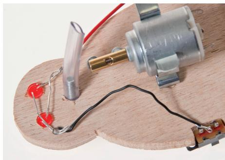
17. Now join from the wire from the switch to the cathode of the LEDs
