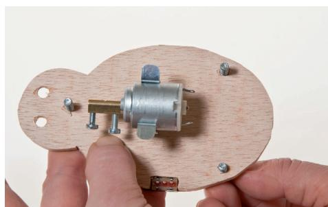
8. Insert the 3 machine screws (12) through the pre-drilled holes
