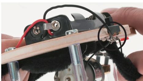
25. The black cable from the battery holder 4 is guided and joined to the right hand connection on the micro switch. Be Careful that this cable does not touch others
