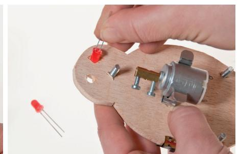
9. Insert the LEDs (9) through the holes in the spider head
