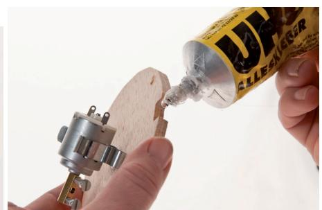
6. Glue the micro switch (5) in the slot as shown. Use an all purpose glue
