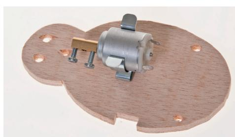
5. Place the motor in the steel clip (7) as shown
