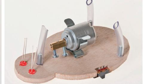
12. Place the tubes over the machine screws as shown. If these are too loose wind a little sellotape around the machine screw thread
