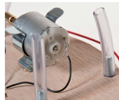
18. Cut a 40-50mm long piece of cable and join it to the minus pole of the motor
