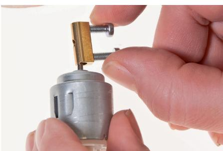
4. Fix the cable joiner (14) on the end of the motor (7) shaft and add the 2 machine screws as shown
