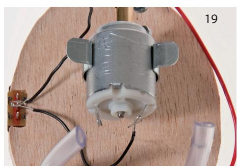
19. Join a cable from the motor (6) to the micro switch (5) this also is joined to the middle connector
