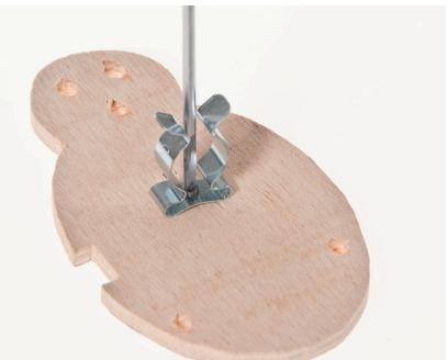
3. Screw (11) the spring steel clip (8) on the centre point of the spider, underneath
