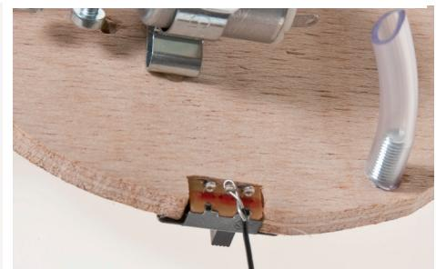
15. Cut a 80 mm length from the cable. Strip the insulation from the ends, join one end to the middle connector on the micro switch .
