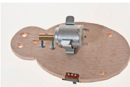
7. Micro switch glued into its slot
