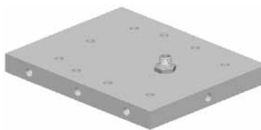
Gear housing base with motor hole and threaded inserts
