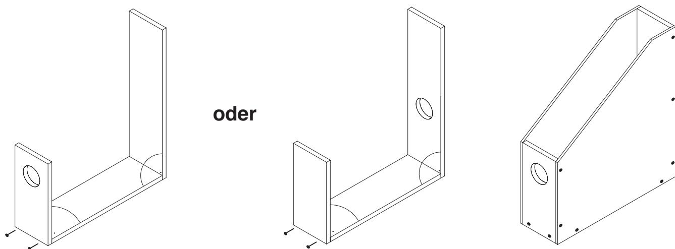
4. Assemble wood parts, glue and nail ( 4 nails ) the bottom and ends as shown.
