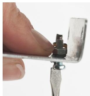
13. Wind the nuts carefully on the machine screws (6) from underneath make them finger tight . If the holes are too tight use a needle file to enlarge them.
