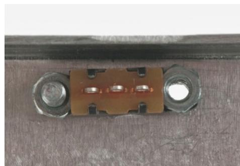
12. Mount the micro switch on the inside of the lid and screw it in place
