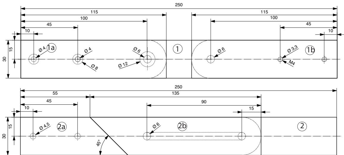
2. With the coping saw roughly saw the curved cuts of parts 1a and 1b according to template A (page 5) and round off with the engineer's file.
