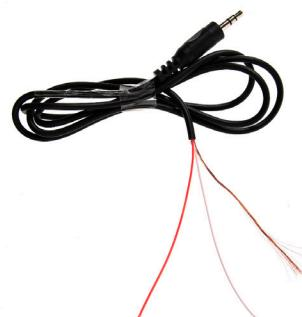
Tie a knot before soldering the cable!
