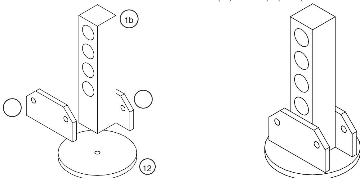
6.3.4 Drill all the pine discs (15) as shown in the diagram.
