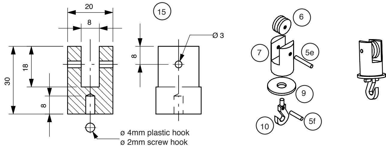
6.5.2 Saw piece 20mm (5e) and 15mm (5f) long from the beech dowel (5) and clean up the ends.
