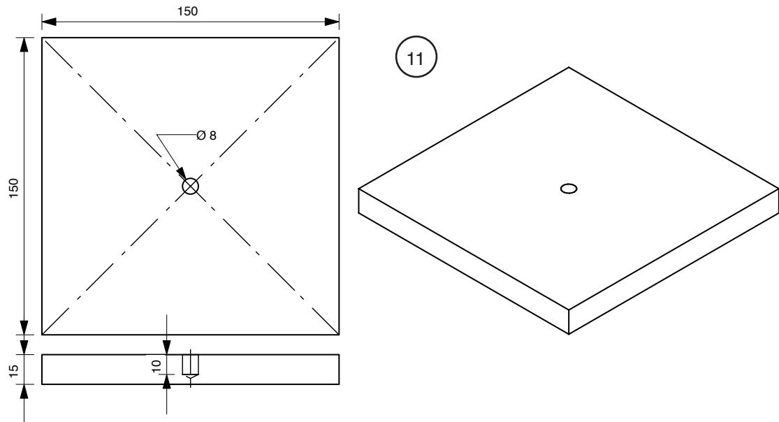
6.4.2 Glue the dowel (14b) from step 6.3.5 in the blind hole in the base (11) and leave to dry. Once set assemble the crane on its base.
