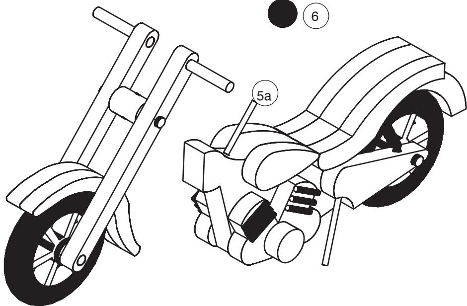
6.3.8 Mark where the steering head (7a) and the mudguard (2e) meet, remove the forks from the frame and glue them in place.
