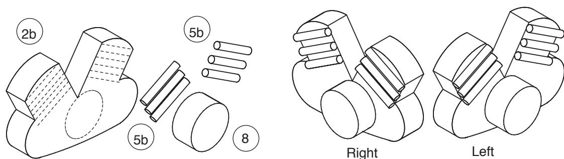
6.2.5 Glue the petrol tank halves (2a) motor block halves (2b) and the seat (2d) left and right on to the frame.
