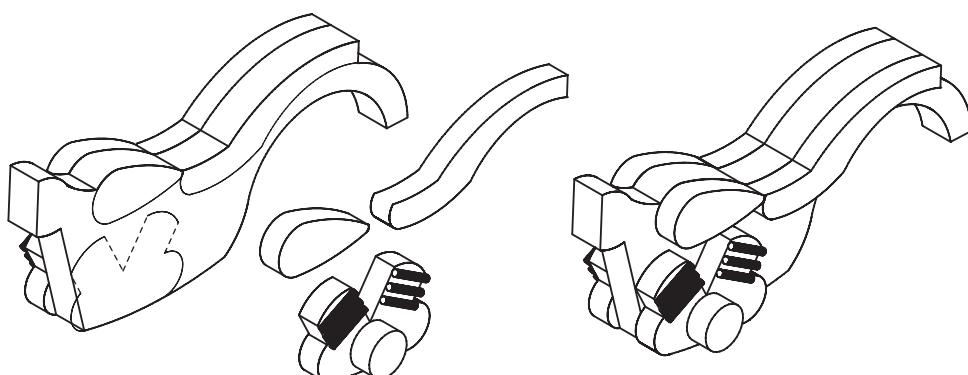
6.2.6 Saw two 45mm long pieces from the dowel (5) and a 50mm long piece ( For the stand) and lightly round the ends.
