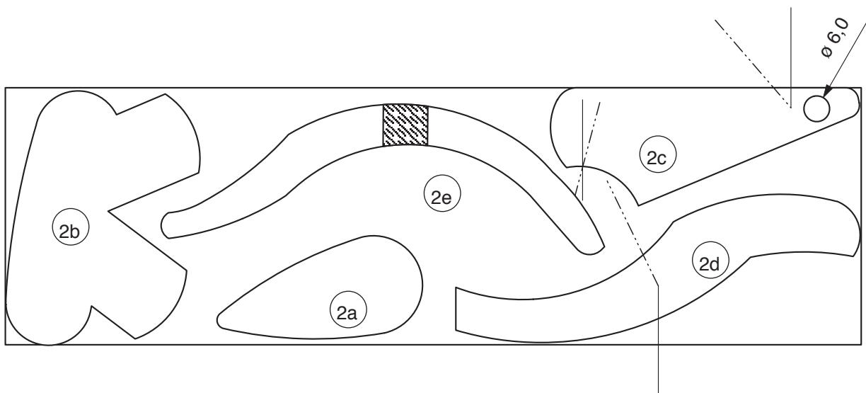
6.2.2 Drill the blind holes, 3mm diameter, 4mm deep in the seat (2c) and the swinging arm (2d). Then drill through the swinging arms a 6mm diameter hole for the rear axle. (See page 9). Finally drill the 4mm diameter x 10mm deep hole for the stand.
