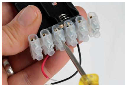
6. Shorten the legs on the 68 Ohm resistor (10) Die Beine des Widerstandes 68 Ohm (10) and screw it between connections 3b+4b (See diagram on page 4)
