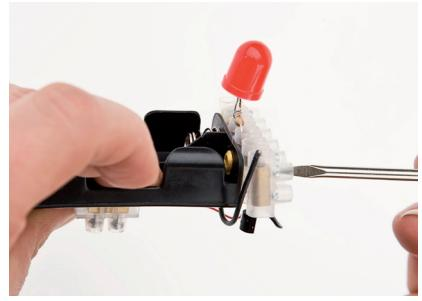
13. The black cable from the battery holder (3) is connected to 6b (see wiring diagram on page 4)
