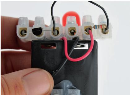
11. Shorten the cables from the battery holder to 50mm and remove the insulation from the ends. Connect the red cable from the battery holder (3) to the (3) to the connection (2a)
