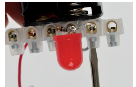
7. Connect the Anode of Jumbo-LED (7) to connection 2b and the cathode (= short leg) to connection 3b.
