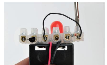
10. Cut a 30cm length from the cable (11) and remove insulation from the ends. Connect the cable between 1a and 4a
