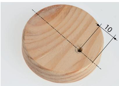
16. Take the wooden wheel (5) and mark out of a hole, 10 mm from the edge. Drill a 2mm hole
