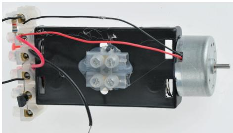
12. Shorten the cables from the motor to 80mm and remove the insulation from the ends. Connect the red cable from the motor (4) to connection 2a, the black lead from the motor is connected to 1a.
