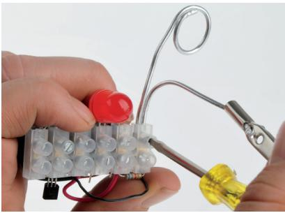
14. File the ends of the feeler (1c) and the grip arm (1b). Connect both to 1b. Connect the second feeler to 5b.
