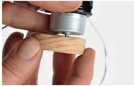
17. Place the wooden wheel on the shaft of the motor (4)
