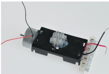
5. Glue to battery case (3) the connection block (6 blocks) On the bottom of the battery case (3) the connection block (2 blocks) and the motor (4) to the opposite side of the cable (12) using a hot glue gun
