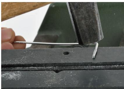
2. Make the 90 degree bend at the end of the leg with a hammer and a hard surface.
