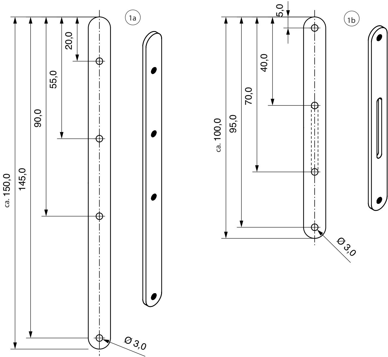
**Note:** Use a pencil to mark the aluminium strip not a scriber, because this would leave marks and scratches in the metal!
