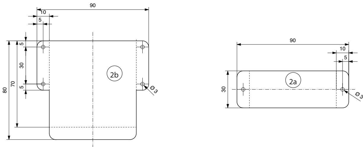
6.2.2 Transfer the bending edges (dashed lines) to the cuttings (2a/2b) according to drawing.
