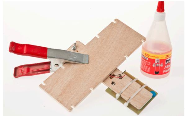
10. Take the black motor cable from and connect it with the middle connection on the switch (Tin an solder the end) From the cable (9) cut a 40mm long piece- remove 10mm insulation form the ends and solder one end to right hand connection on the switch and the right hand connection on the Solar cell (The cable can be carefully soldered or wound around the connector )
