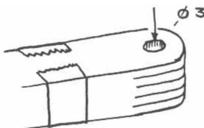
4. The thumb bearing block (5) and bearing (6) are sawn from the pine strip 10 x 20 x 100mm
