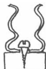
6. Drill the bearing block holes ( 3mm dia and 1.5mm) fix the spring clip (10) using the screw (13) in the 1.5mm hole
