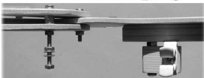
9. Fit the bearing block (6) using the screws (12) and nuts (14) ( see page 3,under the handgrip behind the head)
