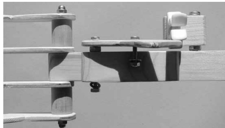
10 Fit bearing block (6) with the machine screw (12) and nut (14) ( see diagram 8) to the handle 5mm from the end
