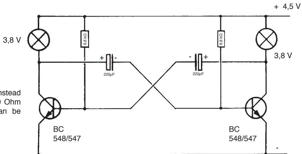
A LED can be used instead of the lamp with a 150 Ohm resistor or a relay can be operated.
