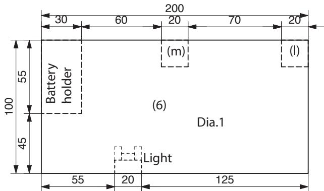
3. Glue the parts (l) and (m) as shown on the base diagram (6) in the marked positions.
