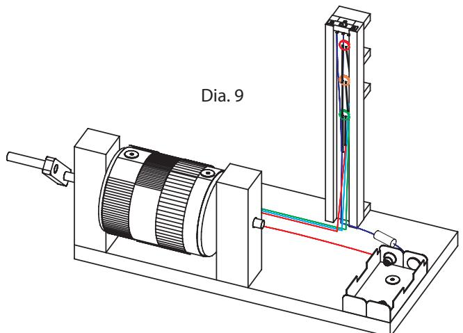
11. Take a ca. 250mm long piece of cable (14) remove insulation from the ends and connect to the anode leg of the red LED (11). Solder the other end to the outer brass strip (See wiring diagram)
