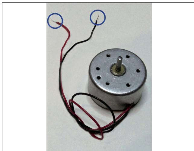
The ends of the motor cables are stripped. You can see the bare metal of the wire where the insulation is missing. This piece of metal must have an electrical connection to the tabs on the solar cell.
