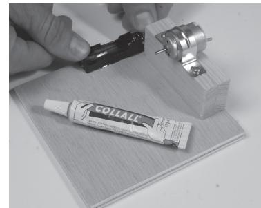
10. Screw the bi-metal holder on the base ,5mm from the edge 20mm in from the end of the base using a screw (9)
