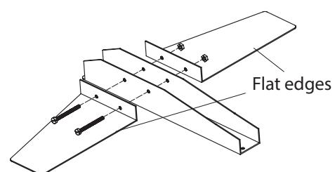
Mount the wings (Parts b/c) as shown using the machine screws (11) M3x35 and nuts (13) to the fuselage body (Part a) (straight edges on the wings point backwards.)
