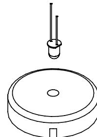
2. Transfer the recess for the switch to the wooden cube (1) according to dimension (see illustration). Then drill through the marking with a Ø6mm drill. Use the warding file to work out the rectangular recess (12 x 6mm). Insert the light-emitting diode (4) in the hole of the wooden wheel as shown. Moreover insert the switch (8) in the recess in the wooden cube (1).
