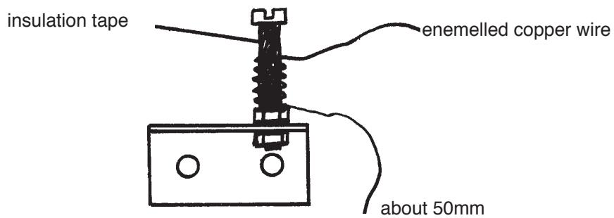
Now add a second set screw and fix it like the first one with two lock nuts. The enamelled copper wire must now continue to be wound on to the second set screw.
