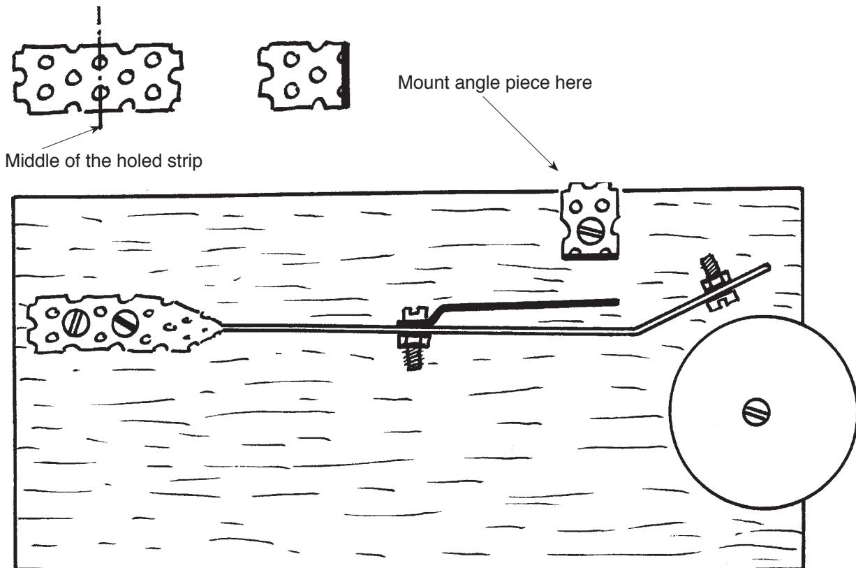
The 3mm long set screw is mounted in the angle piece as shown and locked in position with two nuts, so that it just touches the sprung bronze strip.
