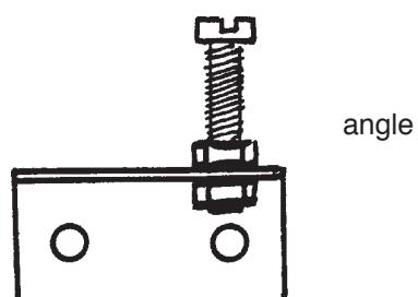
Cover the thread of the set screw with a layer of sellotape or insulation tape, to protect the copper wire from any sharp edges.
