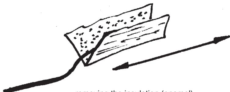
removing the insulation (enamel)
