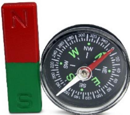
Simple compasses that are stored, for example near magnets, can "lose their orientation". This means that the needle no longer points in the right direction. Rough vibrations or incorrect storage can also irritate the compass needle. In such cases, the compasses are not faulty, but they have to be aligned again.
