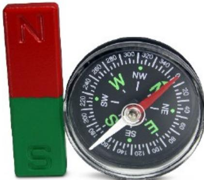
Simple compasses that are stored, for example near magnets, can "lose their orientation". This means that the needle no longer points in the right direction. Rough vibrations or incorrect storage can also irritate the compass needle. In such cases, the compasses are not faulty, but they have to be aligned again.
