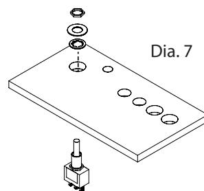
8. Mount the switch (4) in the hole in the shelf (e) and tighten. dia.7
