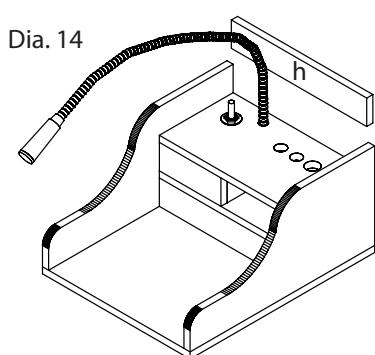
15. Glue the back wall (h)on the shelf (e) as shown and the side parts (b+c) (Dia. 14)
