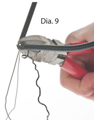
10. Cut the metal casing with side cutters (Dia. 9)
