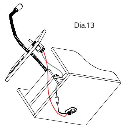
14. Twist together and solder the black cable from the battery lead (6) and the light grey cable from the lamp(3) Solder/ twist the red battery lead to the middle connector on the switch (4) Solder /twist the dark grey cable from the lamp to the outer connection on the switch
