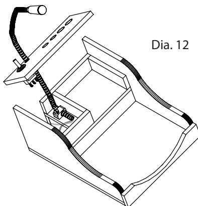
13. Fix the lamp (3) with the clips (5) and the screw (7) as shown (d)
