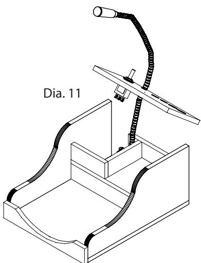
12. Insert the lamp (3) through the 6mm hole in the shelf (e) (Dia.11)
