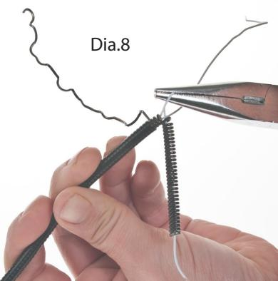
9. On the lamp (3) bend up about ca. 50 mm from the coiled metal casing. Using pliers bend the casing back and insert it through the hole with the cable (s. Dia.8)
