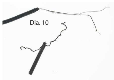
11. Remove the insulation from the cables ca. 10mm, twist the wires together and tin
