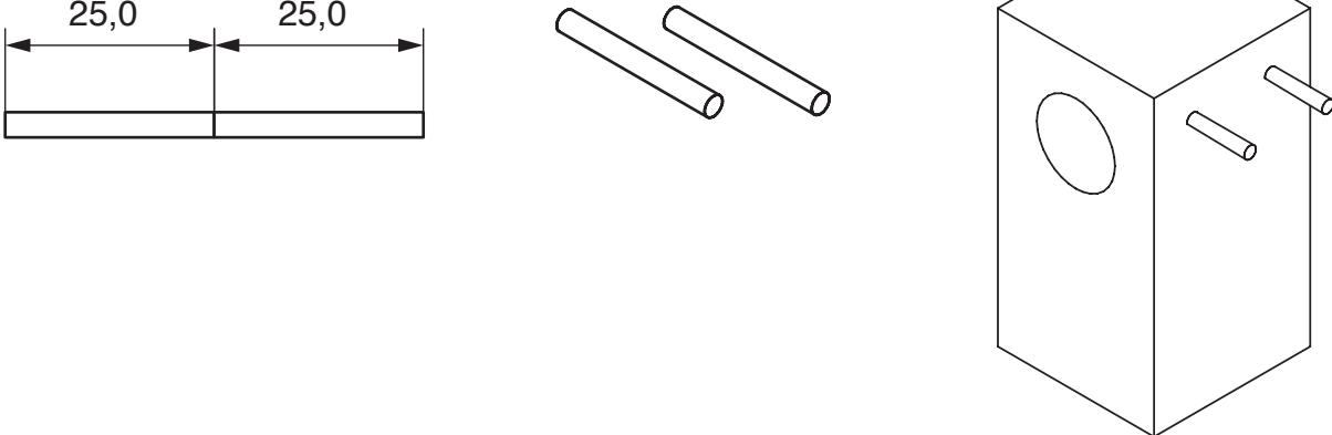
4. Mark out and drill the 3 x 8mm dia blind holes 20mm deep
