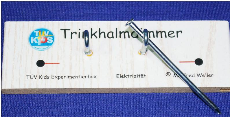
Use a nail as a lever or pliers, then it is easier to screw the ring screws into the board. Take care that they don't come out at the back.
