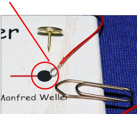
Put a thumbtack through the cable eyelet and the paper clip.
