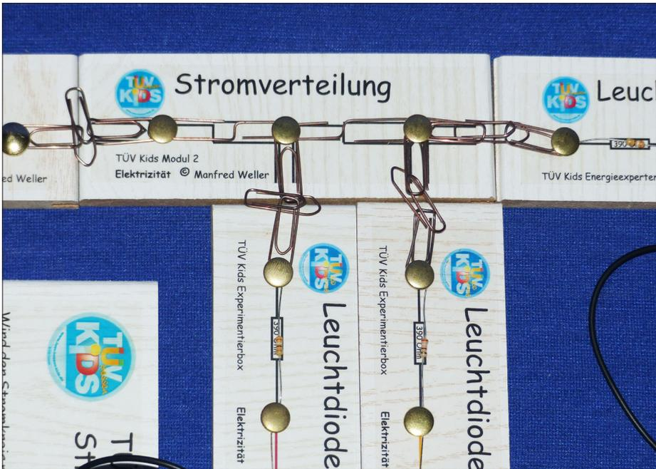
The power distribution helps to save many test lead cables.
