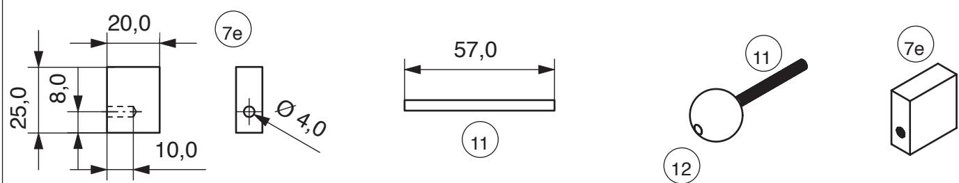
6.1.9 Insert the locking parts (11/12) in the hole in the frame so that the 'Ball handle' is on the mirror side and then glue on the back of the lock (7e).
