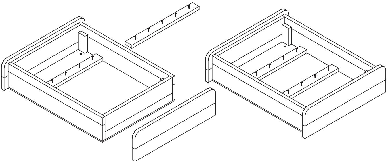
6.2.7 The caps (3/4) are glued in place at either end of the carcase.
