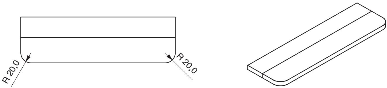
6.2.5 Mark out two strips (1) 10 x 25 x 250mm as shown and insert 5 brass pins (14) as key holders in each marked place.
