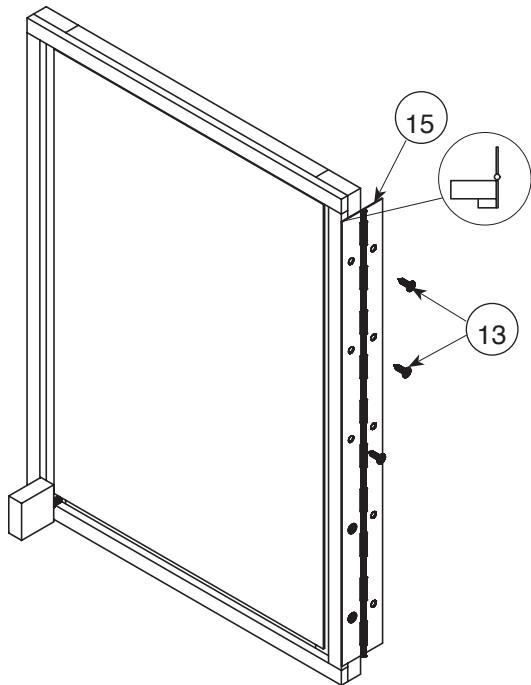
6.3.2 Mount the other half of the piano hinge on the cupboard carcass (As shown)
